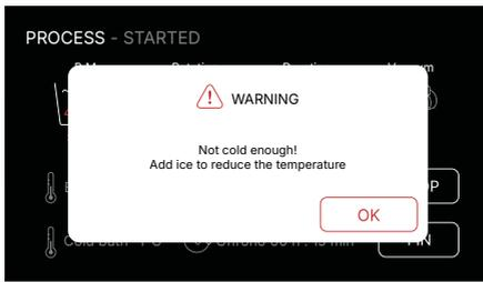
**Warning Cold Bath:** this screen serves as a reminder to add ice to the machine, as the cold bath sensor has detected that the temperature has exceeded 10°C. The warning does not stop any process, but it will appear periodically every 5 minutes, accompanied by a "beep" sound.
