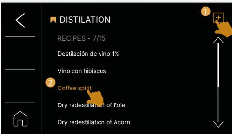
The saved recipes are displayed in this format within each library; in this case, the distillation library is shown. From this screen, you can create new recipes by pressing the button **1** or select a saved recipe **2** to view its summary.
