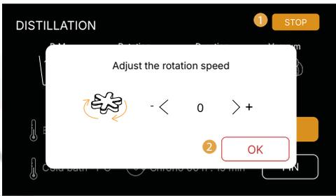
**7 Adjust Rotation Speed:** in this step, you can adjust the motor speed of the paddle using the arrows displayed on the screen, where **0** indicates the **OFF** state of the motor and **9** represents the maximum rotation speed. Once you have adjusted the speed, press **2 OK** to proceed to the next screen.
