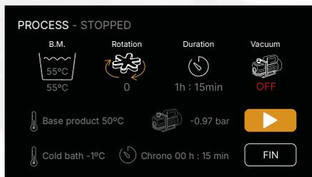
When you press **OK** in the pop-up window, the process will stop and enter pause mode. In this state, the Girovap action screen will only allow you to resume/continue the process or finish it.
