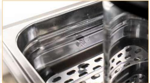
**3 B.M. Temperature:** select the temperature of the water bath, and the water will begin to heat up. On the screen, the current water temperature is displayed gray, and the desired temperature that has been set is shown in orange. The programmable temperature range is from ambient temperature up to 100°C / 212°F. If Girovap is in operation, it will not be possible to modify the bath temperature.
