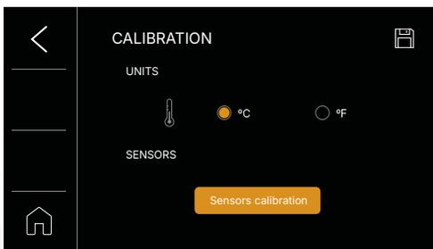
**Calibration:** select the unit of measurement you want to use to display temperature values: degrees Celsius **°C** or degrees Fahrenheit **°F**. If you exit this screen without saving, the machine will return to the previous state upon restarting. If you save, the selected settings will be retained.
