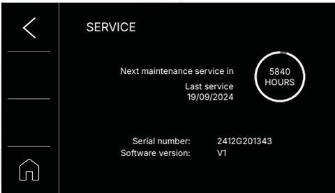
**Service:** displays the expiration controller for the next maintenance service, the date of the last service, and the registration data, along with the software version.
