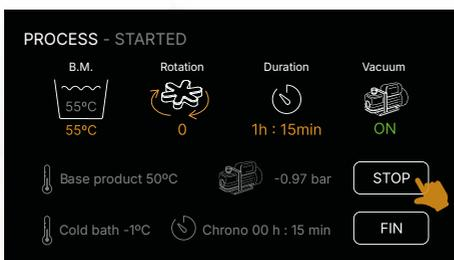
**F STOP:** once Girovap is in operation and you wish to pause the process, pressing the **STOP** button will stop the heating element, motor, stopwatch, and pump. If you are running a scheduled process, the remaining time will also be paused.
