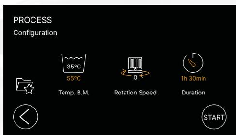
**2 Distillation Configuration:** press each icon corresponding to the parameter you want to modify. For example, if you want to change the temperature, rotation speed, or duration, simply click on the corresponding icon.
