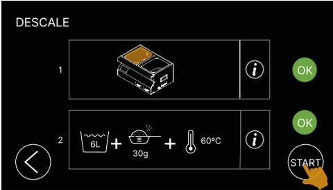
3 Once the previous two steps are completed, press the **OK** button. This will change its status to green. In order to press the **START** button, both **OK** buttons must be green.
