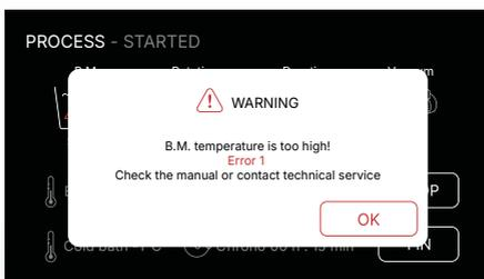
**Warning Error1:** if the heating element does not turn off when the programmed temperature is reached and continues heating, the B.M. sensor will stop the entire machine when it registers a value 11°C above the set temperature. At that moment, the process will become irreversible, and the following warning will appear on the screen.
