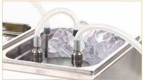
9 **Cold Bath:** secure the condenser coil inside the small clip and add crushed ice or ice cubes, covering the coil and all available spaces as much as possible. To improve the cold transmission, add 200 ml of cold water.
