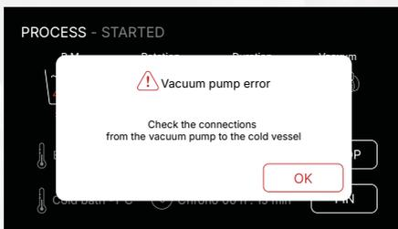
**Vacuum pump error:** this alert is triggered when, during the process, the vacuum drops to an absolute value lower than -0.3 bar. When this screen appears, GIROVAP automatically pauses the process. To resume the process, you must follow the instructions displayed on the screen and ensure that the vacuum conditions are correct before continuing.
