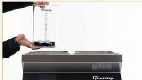
**2 Fill the B.M. Tub:** place the flask vessel with the paddle and Teflon, and fill the water bathtub with water up to at least the level of the upper sensor.
