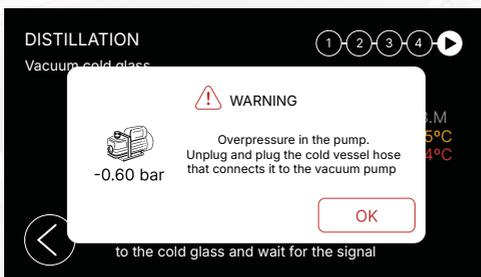
**Warning: Over-pressurized Pump:** if, at the start of a process, Girovap detects that the cold vessel has an absolute value greater than **-0.3 bar**, a warning will be triggered. Follow the instructions displayed on the screen to resolve the issue.
