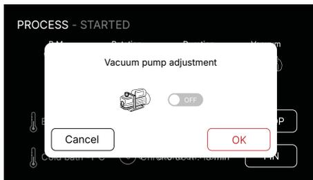
**E Vacuum Pump Adjustment:** unlike the other adjustable parameters, the vacuum pump control can only be accessed through the pop-up window when in an unlimited duration distillation process. Once the window is open, you can turn the vacuum pump on or off.
