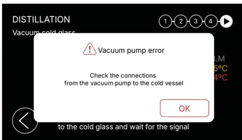
**Vacuum Pump Error:** If it takes more than **1 minute** to create a vacuum in the cold vessel, a **warning** will be triggered. Once validated, the pump will turn back on.
