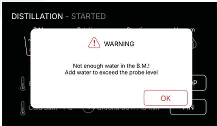
**Water level warning:** this screen appears when the water in the B.M. does not cover the level probe. Check that the beaker flask is in place. If it is and the water does not reach the probe, add more water. Without the flask, as in the descaling process, more water volume will be necessary.
