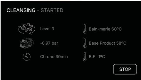
4 When the Sanitization process starts, the heating element will be automatically set to 60°C and will begin heating the water. The rotation will be set to level 3, and the pump will turn on. After the scheduled 30 minutes, the process will successfully complete.
