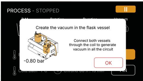
15 Create the vacuum in the flask vessel
