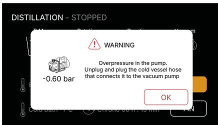
**Over-pressurized Pump:** this pop-up window appears when GIROVAP detects that the content intended for vacuuming has an absolute pressure value greater than **-0.3 bar**. Follow the steps displayed on the screen to resolve the issue.
